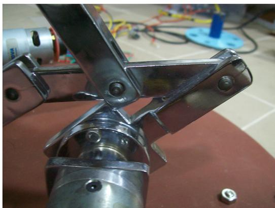
(b) Fork type arrangement of links connected by a pin
