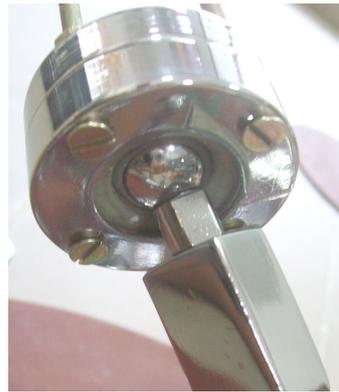
(a) Spherical joint designed in-house
